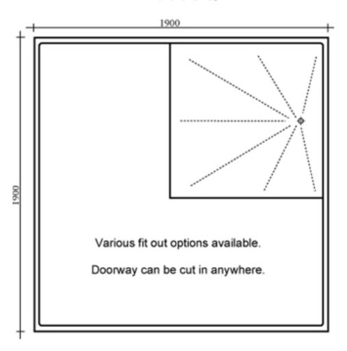
FP1900SQ overall height is 2250 mm. This unit has an integral ceiling panel.
