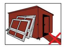
Handle and stack frames carefully on site. Stand them upright on their sills (bottom of the window as installed), raised off the ground on pieces of timber or bricks. Stand them against a flat, vertical surface such as a shed and tie firmly in position.
